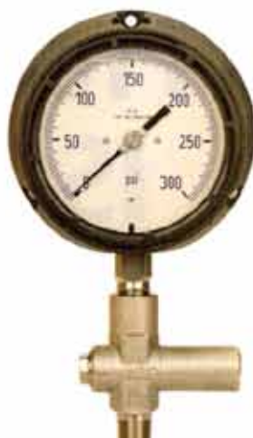
Figure 3. Pressure gauge with overprotector
