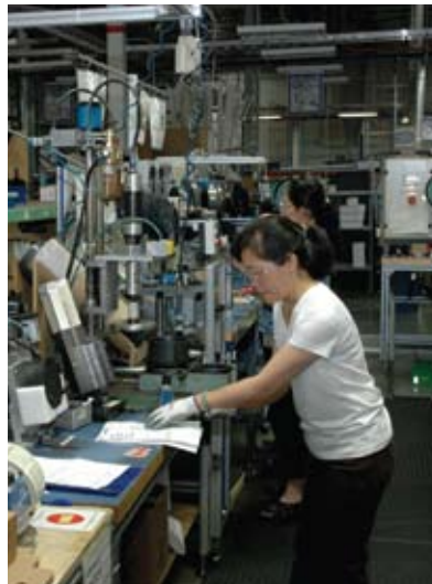
Employees work within U-shaped manufacturing cells that include all necessary production tasks at the Lawrenceville, Ga., facility for WIKA Instrument Corp.
